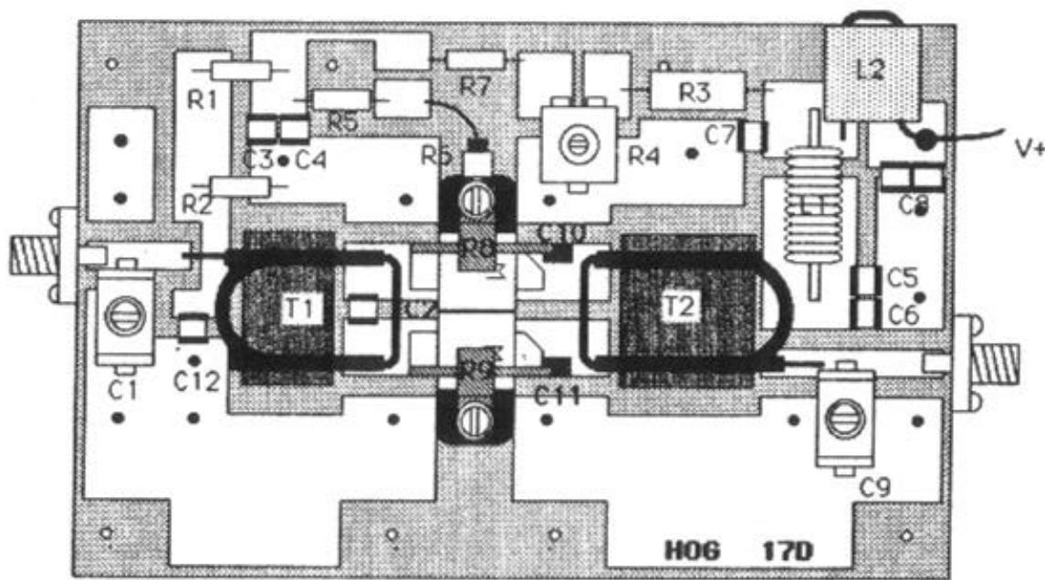
Fig. 1 component layout diagram of 300 W. VHF amplifier
